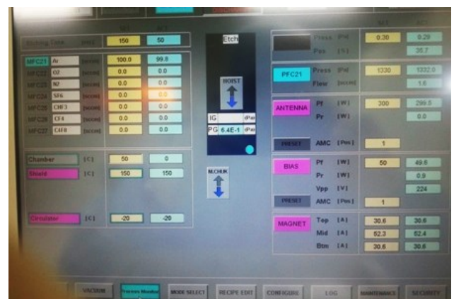
Fig. 2 Condition of Plasma etching.
