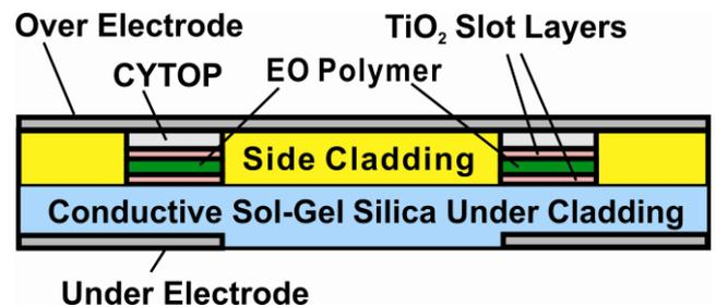
Fig. 1 Cross-sectional view of the MZ EO polymer/TiO<sub>2</sub> multilayer slot waveguide modulator in the active region.
