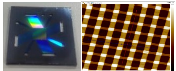
Fig. 1 Device photograph (left) and AFM image of the ANA nanochannels (right).
