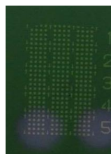
Fig. 1: Patterned electrode on GaAs wafer
