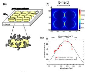
Figure 1(a) A schematic illustration of gold nanostructures array conjugated with crystal violet molecules. (b) Electromagnetic field intensity distribution of gold nanostructures with a small nanogap by FDTD simulation, (c) SERS enhancement factor as a function of incident wavelength.
