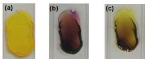
Fig. 4 Photographs of thin films of compound 2. (a) as deposited (b) after polymerization (c) after treatment with hydrazine solution.
