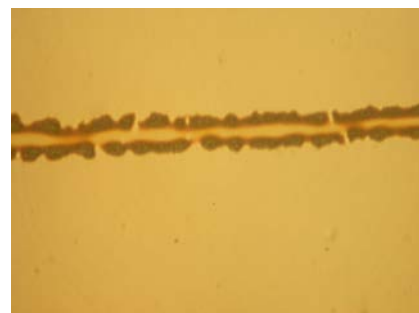
Fig.2 The microscope image after three coat and baking works. Broken and forked structures are observed.
