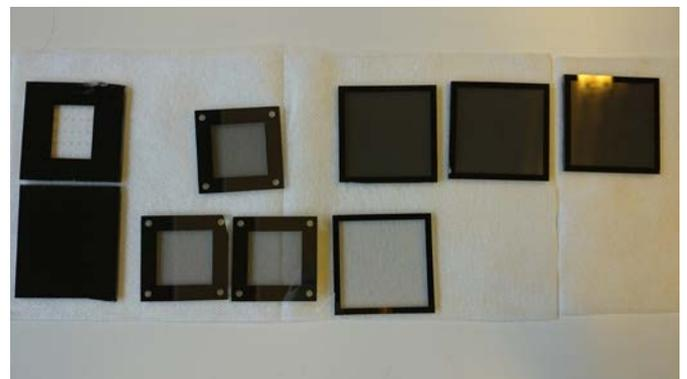
Fig. 2 Samples of diced photo-mask
