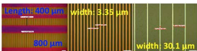
Fig. 2 Photo images of the micro-/nano-patterns on the photomask.
