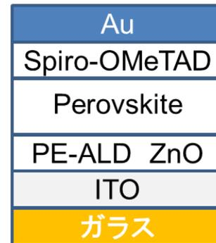
Fig.1 Structure of the cell.
