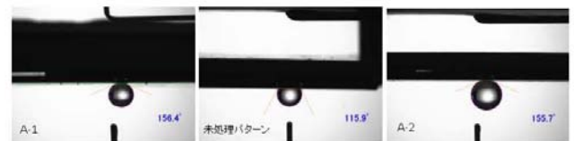
Fig. 3 Images of contact angle measurement of the samples.
