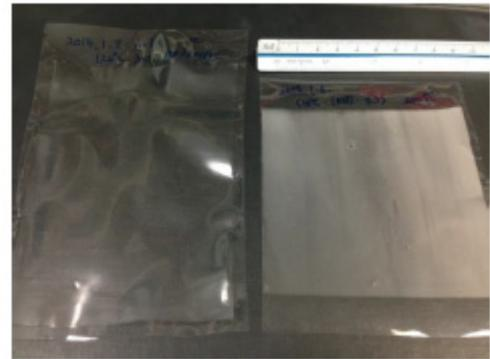
Fig.2 Films replicated by 100- and 200- $\mu\text{m}$ -thick metal molds.
