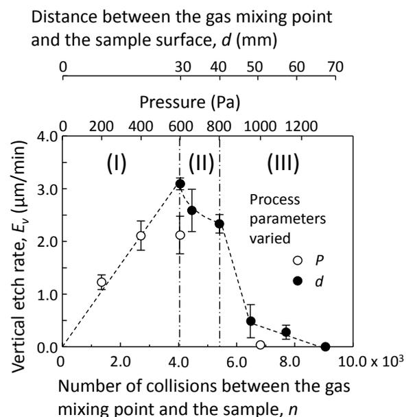
Fig. 1 Relationship between the vertical etch rate,  $E_V$ , and the number of collisions between the gas mixing point and the sample,  $n$ . Two experimental parameters were varied, one was the pressure,  $P$ , and the other was the distance between the sample and the mixing point,  $d$ .
