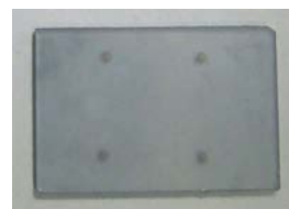
Figure 3: Photograph of electrode on new oxide semiconductor substrate
