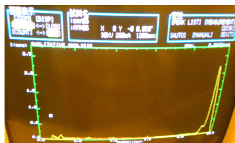
Fig. 3. TXRF spectrum of GaN substrate after immersed in BHF for 10 min.
