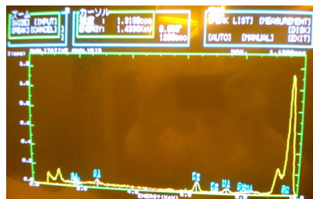
Fig. 2. TXRF spectrum of GaN substrate exposed in draft chamber for 60 min.
