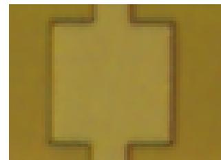
Fig.2 Optical microscopy image of fabricated photo resist pattern on diamond substrate.
