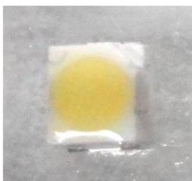
Fig. 1 LED chip with newly developed Ce-based fluorescent material.
