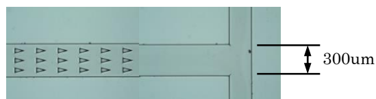
Fig.2 Micro Fluid Channel Resist Pattern.
