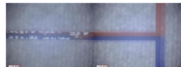
Fig. 3 PDMS Micro Fluid Channel.
