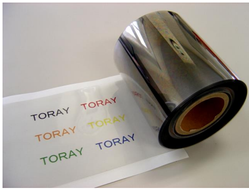
Fig.1 Photograph of conductive transparent DWCNT film prepared by a role-to-role method
