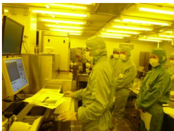
Fig. 1 Training of high speed maskless lithography system to draw diffractive optical element pattern
