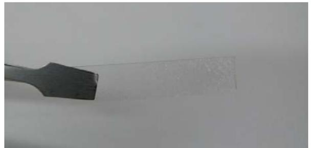
Fig.1 Photograph of glass substrate coated with  $SiO_2$
