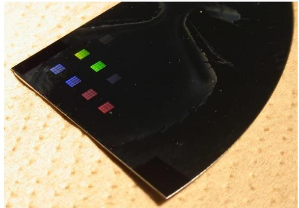
Fig. 1. Fabricated Micro Lines & Spaces on a wafer
