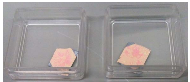
Fig.1 Photograph of the sample covered with an Au film by sputtering on the Si board with resin.
