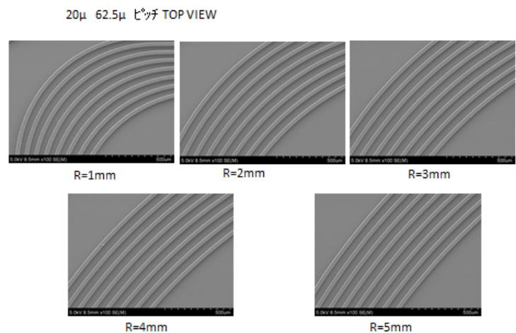
Fig.1 SEM Images of Bend Waveguides.
