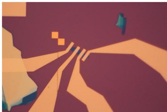
Fig. 1 Microscopic image of an MoS<sub>2</sub> transistor.
