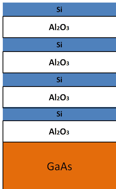
Fig.1 Cross-section of the dielectric multilayer reflector.
