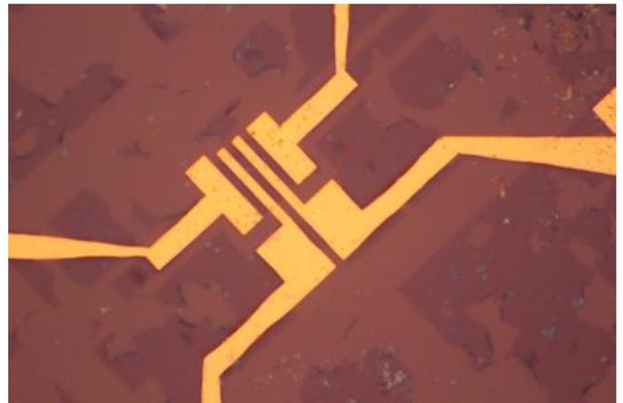
Fig.1 4 terminal electrode pattern on isolated CVD graphene.
