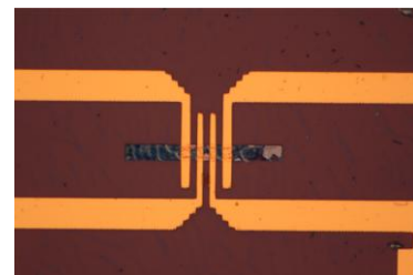
Fig.1 Four terminal electrodes with graphene.
