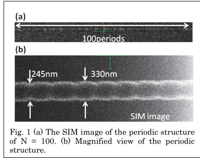
Fig. 1 (a) The SIM image of the periodic structure of  $N = 100$ . (b) Magnified view of the periodic structure.
