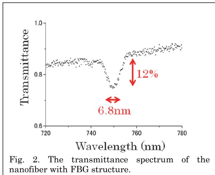
Fig. 2. The transmittance spectrum of the nanofiber with FBG structure.
