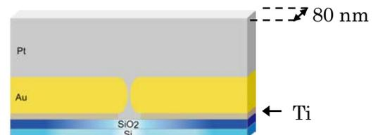
Fig.1 Schematic image of nanogap electrodes after FIB milling
