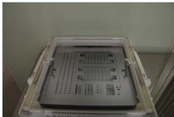
Fig. 1 Photograph of reticle for Si fluid channel microfabrication.
