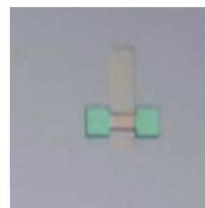
Fig.1 Optical microscope image of a InGaAs TFET
